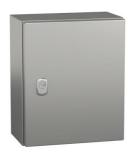
Wall mounted enclosure, Spacial S3X, stainless steel 304L, plain door, 300x250x150mm, IP66
